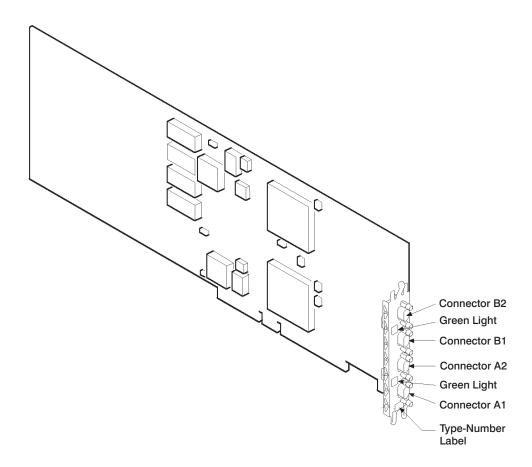
The SSA links must be configured as loops. The loop is connected to the internal connectors at the SSA adapter card. These connectors *must* be a valid pair (that is, A1 and A2, or B1 and B2); otherwise, the disk drive modules on the loop are not fully configured, and the diagnostics fail. Operations to all the disk drive modules on a particular loop can continue if that loop breaks at any one point.
